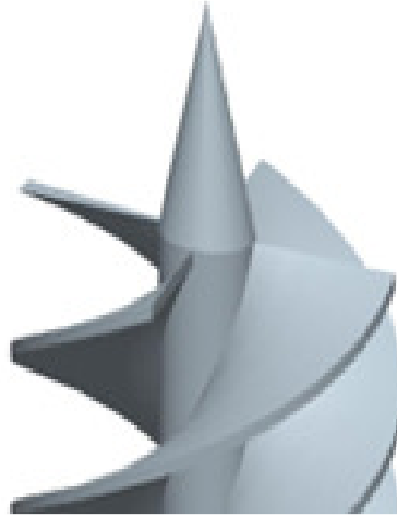
Figure 46. Swirl Inducing Device: Quadruple Ribbon Cylindrical Helicoid Attached to a Cone.
